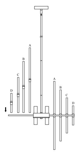
1. Put the glass bars A, B, C, D into the slot, and then twist the bulb to power on.
